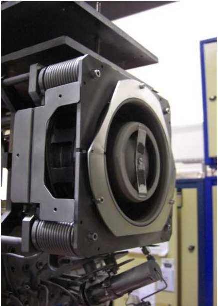
5 kW PPS-X000 thruster (Safran) mean diameter 12.5 cm
